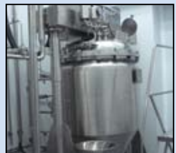
750 ℓ Raise/lower contramix vessel
