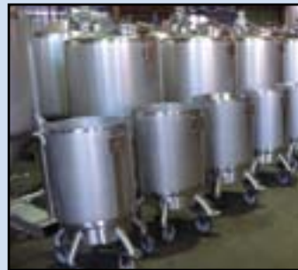
100 ℓ Mobile premix tanks ready for factory acceptance test
