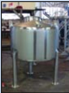
500 ℓ Cold water tank cleaned and complete
