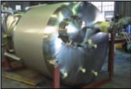
3000 ℓ Manufacturing vessel on cradle ready for transport
