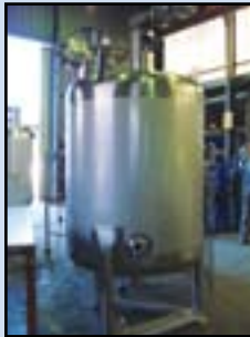
1500 ℓ Manufacturing vessel cleaned and completed
