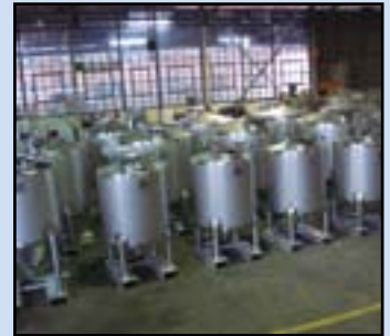
1500 ℓ and 500 ℓ Portable storage vessels ready for factory acceptance test
